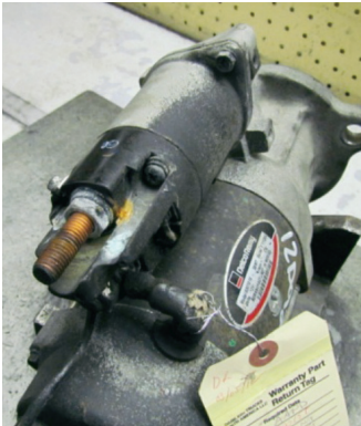
Missing IMS switch
