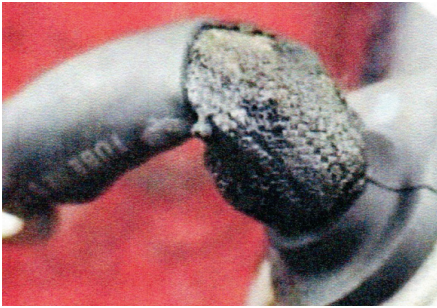
Strap damaged from heat
