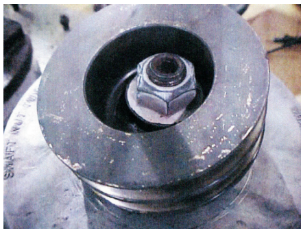
Examples of loose pulley damage on external fan type alternators
